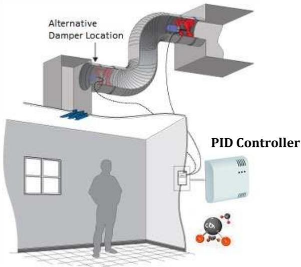
$$u_{PID}(t) = k_p e(t) + k_i \int e(t) dt + k_d \frac{d}{dt} e(t)$$
